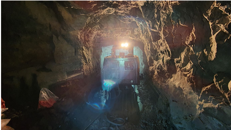
Figure 6. Jumbo working on the 376 m level
